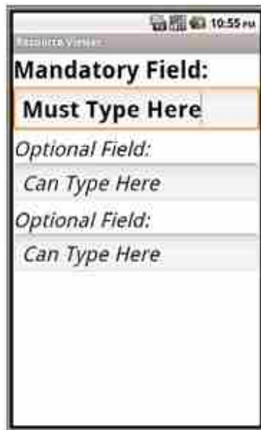
Figure 7.6 : A layout using two styles, one for mandatory fields and another for optional fields.
