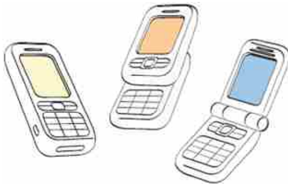
Figure 1.3 : Various mobile phone form factors : the candy bar, the slider, and the clamshell.
