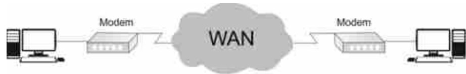
Fig. 4.14 : A Modem Connection through a WAN Handles Analog and Digital Signals
