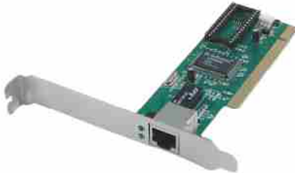
Fig. 12.1 : NIC Card a Hardware Chip to Connect Device in Network
