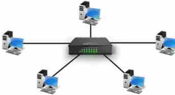
Fig. 13.2 : Hub Device Connected with n Number of Device
