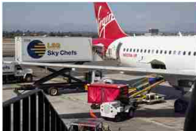
Example of Catering Being Uploaded in the Aft Galley
