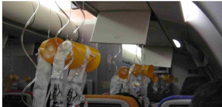
Example of Oxygen mask falling automatically during decompression from the PSU
