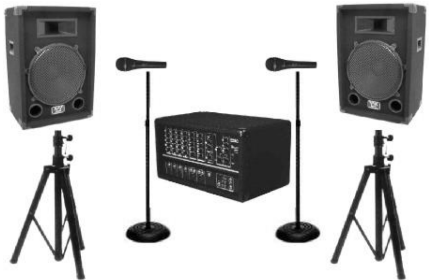
Fig 1.17: PA System Courtesy Google
