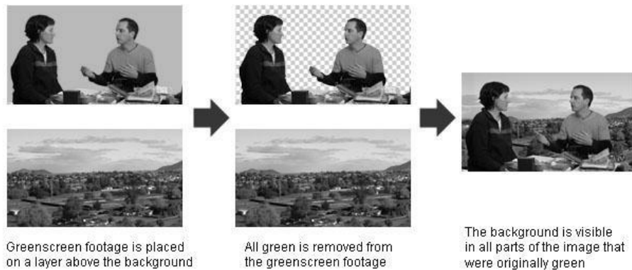
Fig. 6.2: Visual representation of how chroma work and final output
