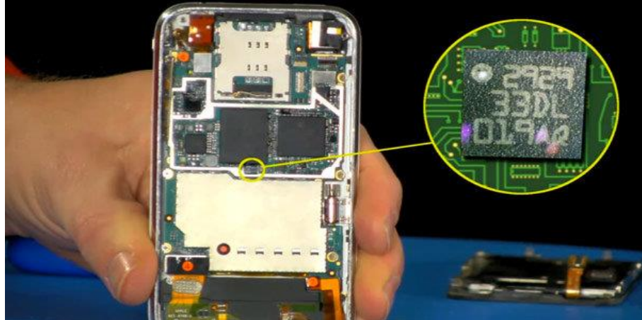
Figure-28 Accelerometer of smartphone [5]
