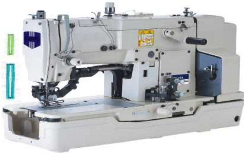
Buttonhole machine (fig-10)
