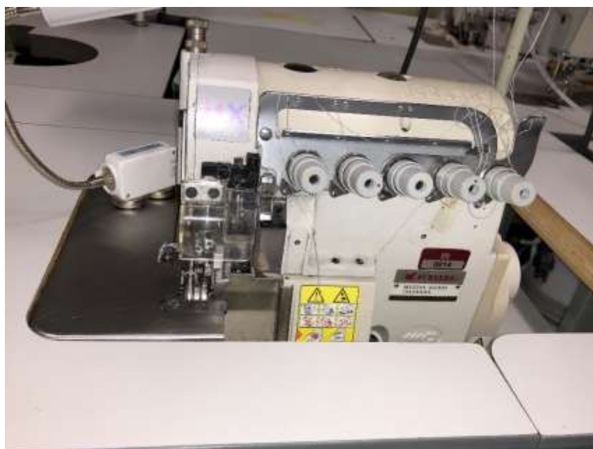
Safety stitch machine (fig-8)
