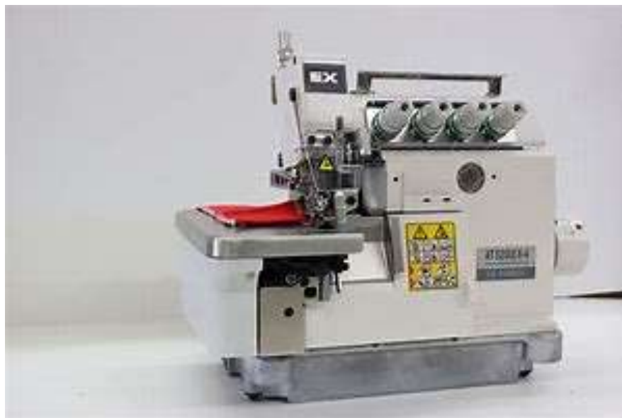
Over lock stitch machine (fig-7)
