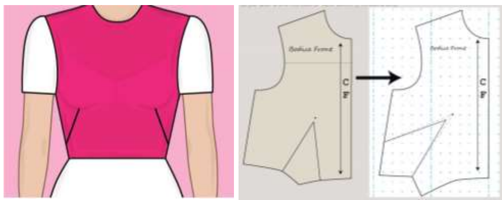
Fig: 5 Pattern with side-seam dart
