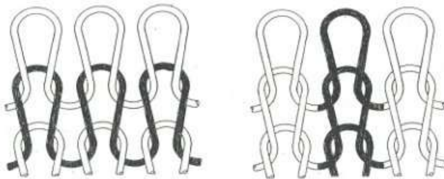
Fig. 5: Arrangement of Course and Wales in knitted fabrics Source: http://www.tikp.co.uk/knowledge/technology/knitting/principles/
